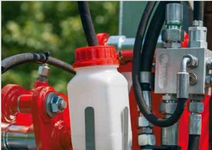
The 6 bar pressure limiting valve protects the engine of the trimmer from pressure peaks in the return flow, as well as from operating errors.
