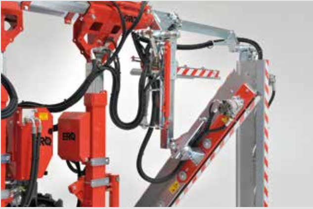
Impact protection on vertical and horizontal cutter beams by means of gas springs, automatic return.
