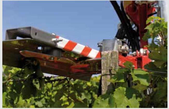
Impact protection on vertical and horizontal cutter beams by means of gas springs, automatic return.
