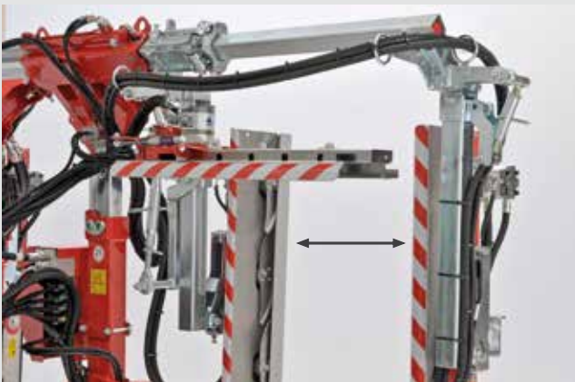
Manual cutting-width adjustment (10 cm - 85 cm).
