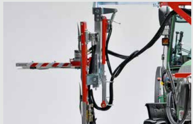
Hydraulic cutting-height adjustment, 40 cm
