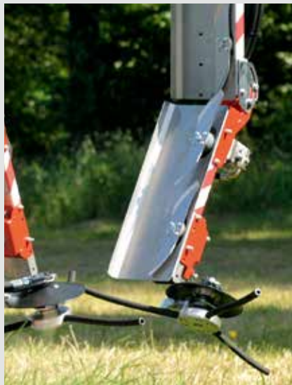
Shoot lifter on lower cutter beam with two blades
