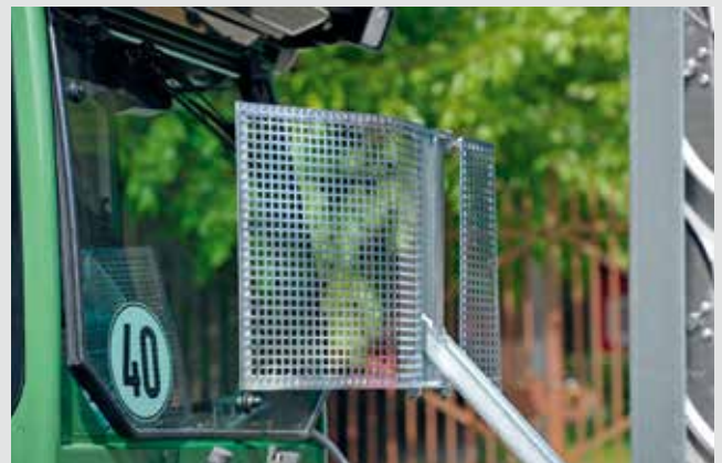
Cut protection for Trimmer on trolley, complete and mounted
